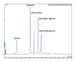
As can be seen from the above HPLC chromatogram in which equimolar quantities of tyrosol, oleocanthal, oleacein, oleuropein aglycon and ligstroside aglycon have been tested, it is obvious that they give a completely different area and therefore concentration in olive oil. This is a very critical mistake because all the phenolic ingredients of olive oil that contain the moiety of hydroxytyrosol (like oleacein, oleuropein aglycon and oleomissional) have almost double
